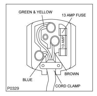
Connect the green and yellow (earth) wire to the terminal in the plug which is marked with the letter 'E' or the earth symbol ( ) or coloured green and yellow.
